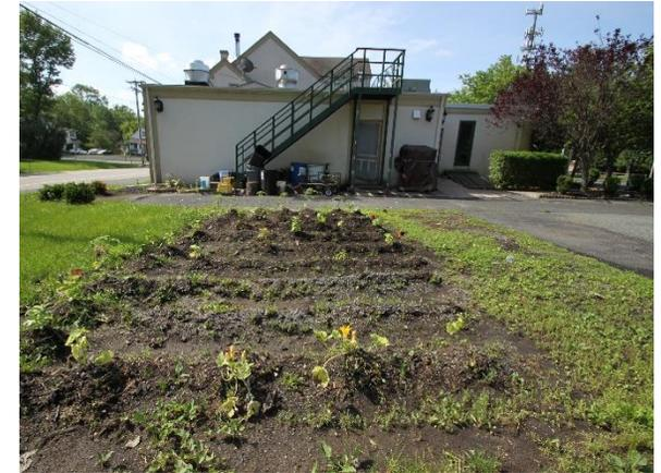
Rainwater on the site drains onto the road and pools at the entrance. Parking spaces can be replaced with porous asphalt to infiltrate stormwater. A cistern can be installed north of the building to harvest rainwater to be used by the existing garden. A bioswale and rain gardens can also be installed to capture, treat, and infiltrate runoff. A preliminary soil assessment suggests that more soil testing would be required before determining the soil's suitability for green infrastructure.
