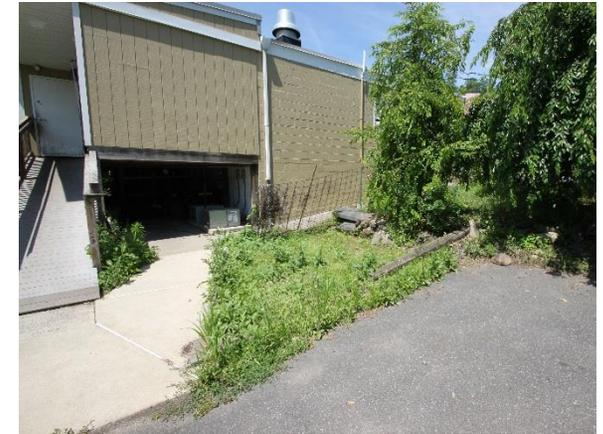
There is a detention pond to which appears rainwater drains. There is an opportunity for rain gardens to be built east of the building to capture, treat, and infiltrate runoff and the parking lot. Parking spaces north of the building can be replaced with porous asphalt to capture and infiltrate runoff. A preliminary soil assessment suggests that the soils have suitable drainage characteristics for green infrastructure.
