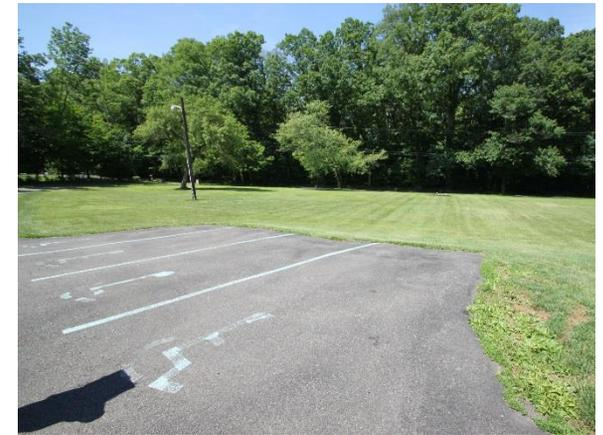
Rainwater drains into the lawn area west of the building. A rain garden can be built on the lawn to capture, treat, and infiltrate roof and parking lot runoff. The parking spaces southwest of the building can be replaced with porous asphalt to allow stormwater to infiltrate. A preliminary soil assessment suggests that the soils have suitable drainage characteristics for green infrastructure.
