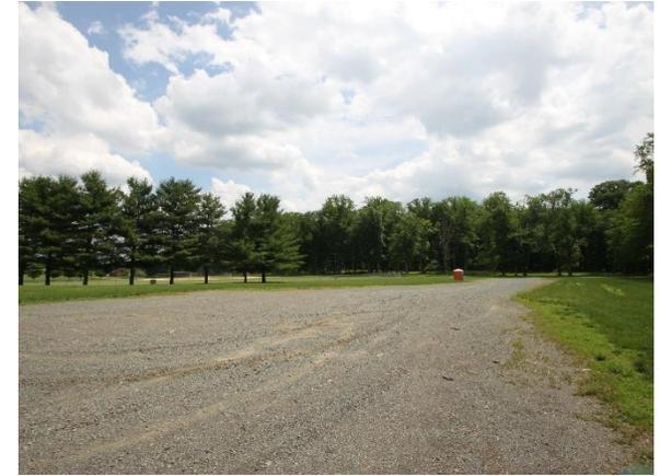
Heavy pooling occurs in the parking lots south of the tennis courts. Rain gardens can be installed along the lots to capture, treat, and infiltrate runoff, which would help remediate this issue. Additional rain gardens can be installed to manage roof runoff. A preliminary soil assessment suggests that the soils have suitable drainage characteristics for green infrastructure.
